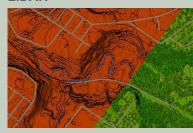
LiDAR is a remote-sensing technology that produces surface models from measured laser pulses emitted from a
