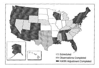
Forty states now have HARNs completed, underway, or scheduled for the near future. Wisconsin was among the first states to implement a high precision network adjustment. The Wisconsin High Precision Geodetic Network (WHPGN) resulted in the NAD 83 (91) datum adjustment for Wisconsin.
