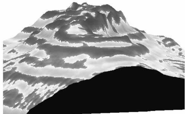
A portion of a 10-meter DEM as displayed in 3-D Mapper. The profile curvature of the terrain has been calculated and mapped on the surface. The dark areas are places where the curvature of the surface along a vertical north-south plane is convex, and the light areas are concave. The software can also calculate curvature along horizontal planes.
