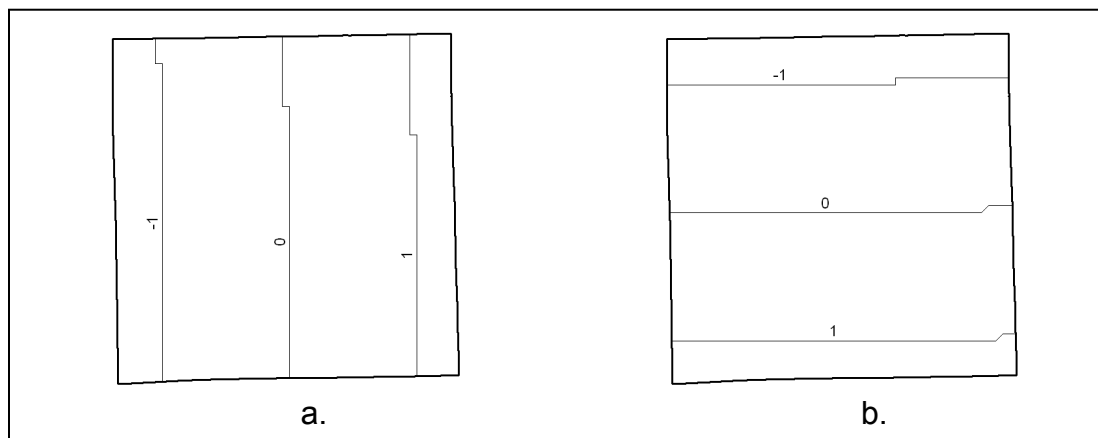
Isoline Maps of a) Easting (X) Shift and b) Northing (Y) Shift (in Millimeters) for Walworth County
