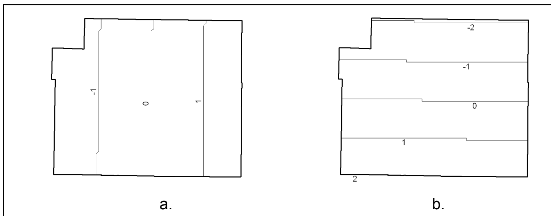
Isoline Maps of a) Easting (X) Shift and b) Northing (Y) Shift (in Millimeters) for Chippewa County
