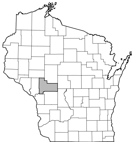
The *Jackson County Official Projection* does not use an enlarged ellipsoid and is instead referenced to the GRS 80 ellipsoid. It is based on a transverse cylindric projection using the following parameters:
