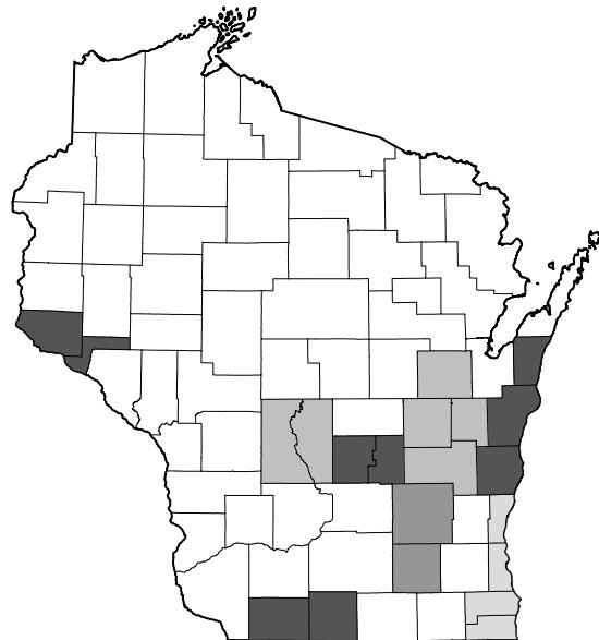
Adjoining counties shown with a common shade share a single coordinate system; unshaded counties each have a separate coordinate system.
