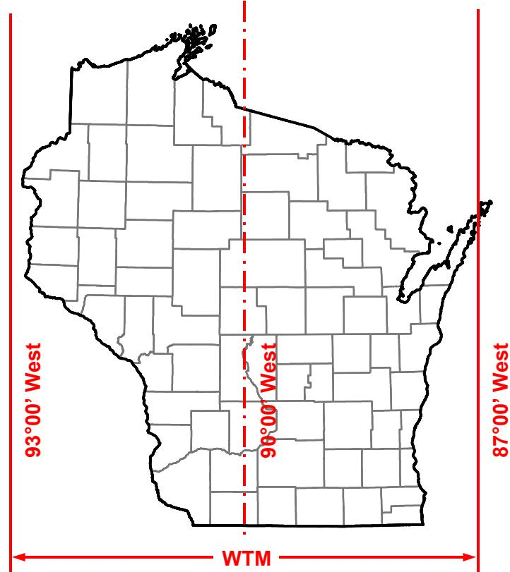
WTM is defined for NAD 27 and NAD 83. A distinct "shift" of approximately 13 miles in northing and easting was introduced to the NAD 83 parameters to more easily distinguish the coordinate values:
