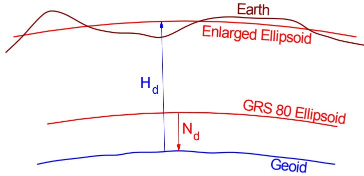
Since the semimajor and semiminor axes are changed, so are the flattening and first and second eccentricities. These can be computed from the ellipsoid equations shown in **Section B.1**. The new ellipsoid parameters must be used in projection equations to convert coordinates between County and Geodetic (or State Plane, UTM, WTM) Coordinates which in turn are referenced to the GRS 80 ellipsoid.
