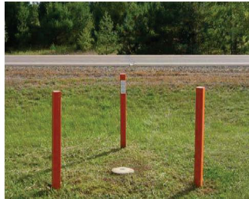
Figure 4 – WisDOT HMP GPS station
