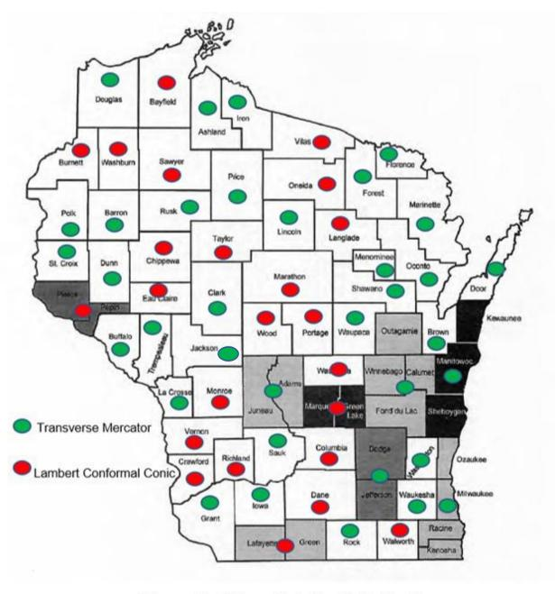
Wisconsin's 59 Low-Distortion Projection Zones: 24 Lambert Conformal Conic and 35 Transverse Mercator
